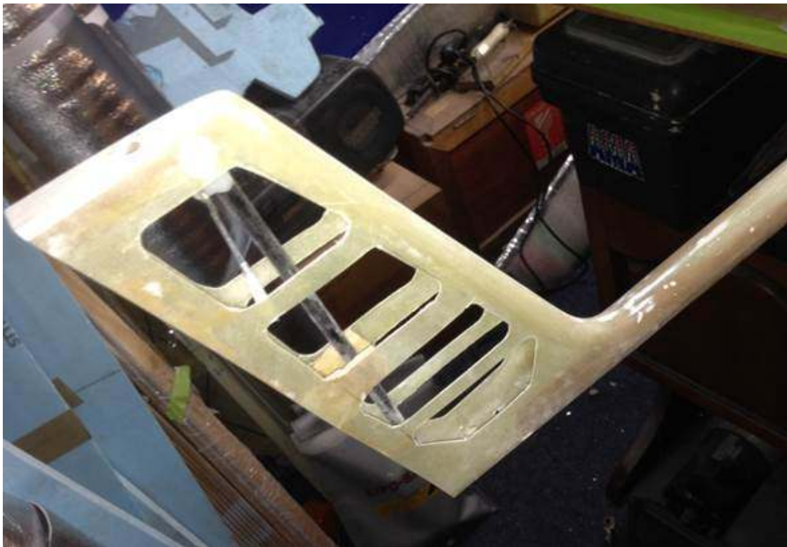
Fin made narrower and with cut-outs to reduce weight.
