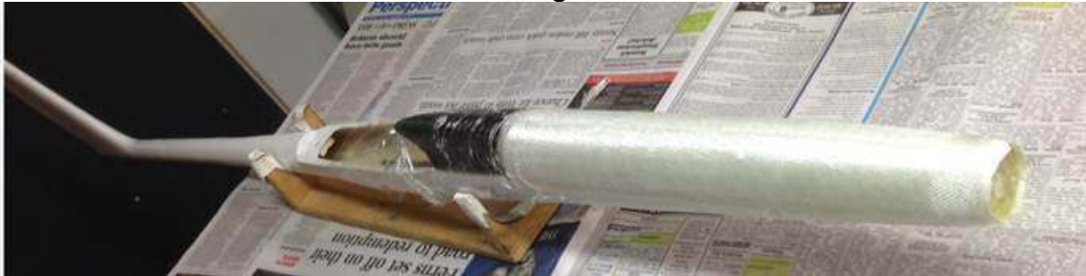
3 layers of 4 oz glass on with light contact adhesive spray to hold it all in place.
