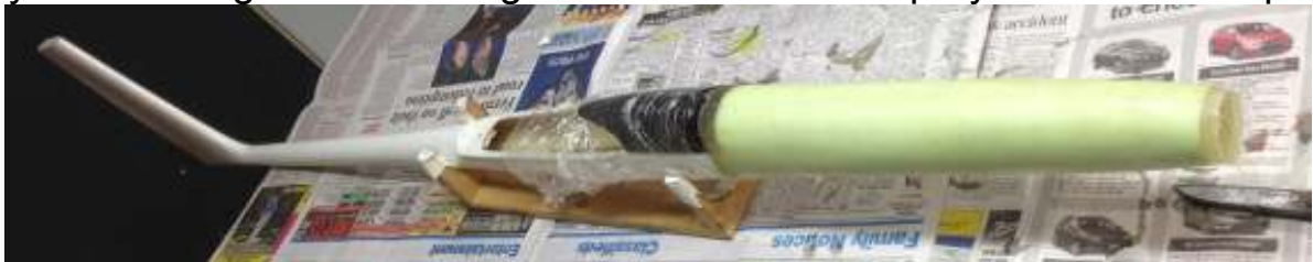
Resin scraped through. Green foam colour shows it is wet right through.
